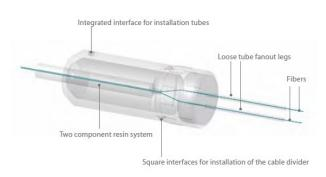
Installation protection: The package of application specific "variable" legs is a not pull resistant dust-proof foil tube.
